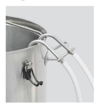
3. Check which hose is connected to the immersion chiller where the coil goes straight to the bottom (see image below). On the other end of that hose, attach the tap adapter and push the final clamp onto the end.
